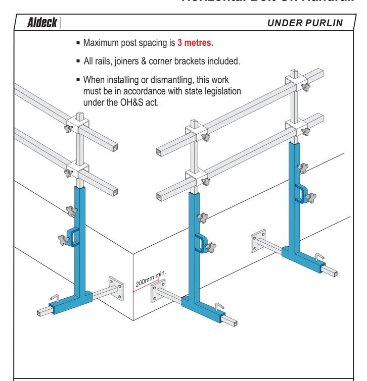
The Aldeck Bolt On System can be attached to many different structure types.
