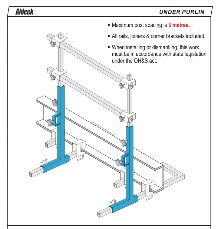
The Aldeck Alternate Beam Connecting System
