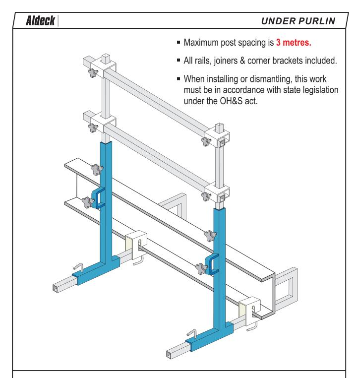
The Aldeck Alternate Beam Connecting System
