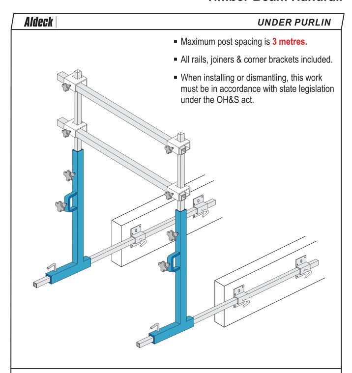
The Aldeck Alternate Perimeter System with Timber Beam Connectors
