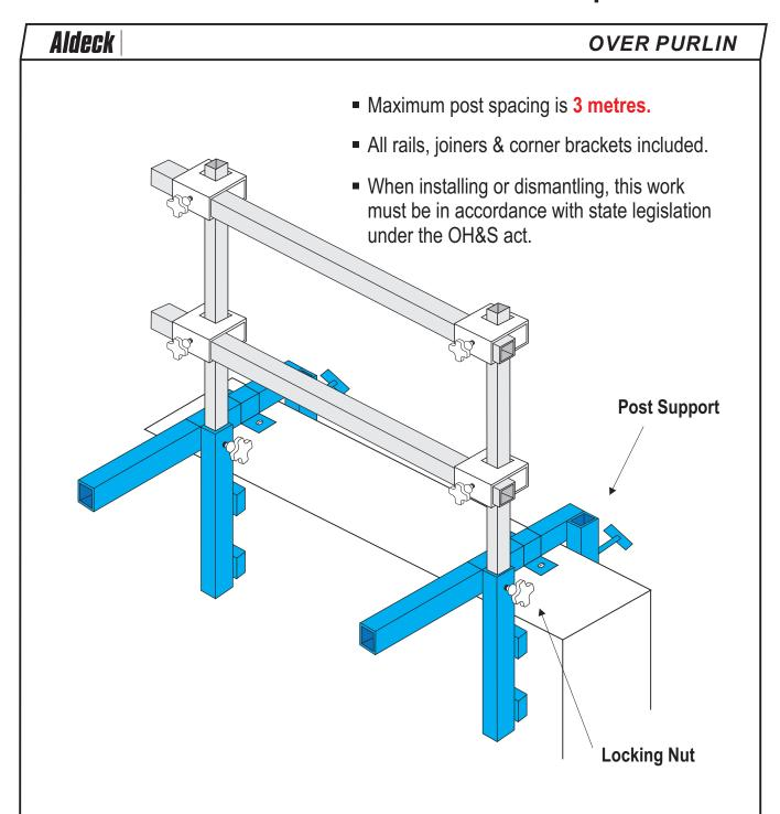
Our new and improved clamp on bracket, firmly connects to panel walls or hobs.
